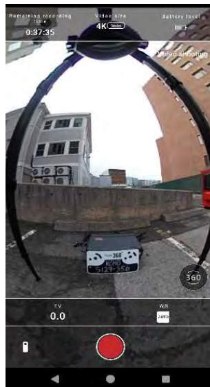
Figure3: Make certain the Project Board is in a fixed position and clearly visible in the camera frame before stopping the recording process.
