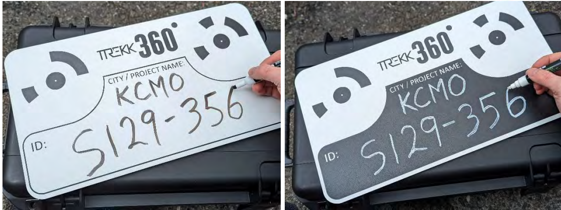
Figure 1: Write the Structure ID on the Project Board in the space provided. One side of the board is meant for a dry-erase marker, and the other side is meant for chalk. Place the Project Board in a stable, fixed location that is clearly visible in the camera frame.
