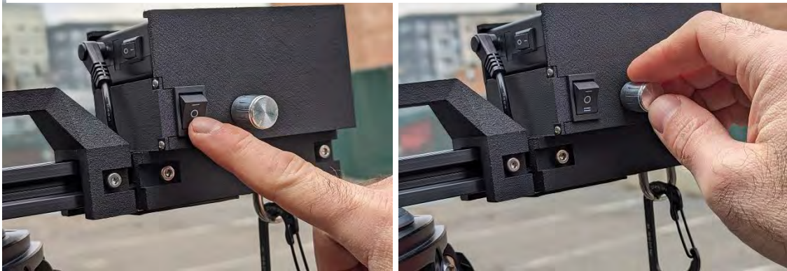
Figure 2: The Rocker Switch (left) determines ascent or descent of the camera. The Speed Control Knob (right) adjusts the speed of the ascent/descent.
